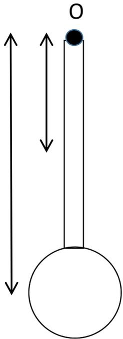
$$I_O^{Barra} = I_{CM}^{Barra} + M_B d_{CMB/O}^2 = \frac{2m(L)^2}{12} + 2m\left(\frac{L}{2}\right)^2$$
